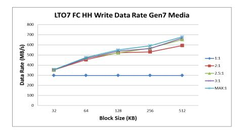
The half-height form factor drive provides similar streaming performance as compared with the full height drive.
