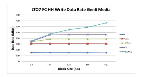
The half-height form factor drive can read and write LTO Gen 6 media with similar rates as compared with the full height drive with LTO Gen 6 media.
