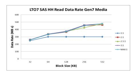
The following charts show the LTO-7 SAS half height tape drive performance when writing or reading LTO gen6 media with data that compresses uniformly at ratios 1:1, 2:1, 2:5:1, 3:1 and maximum (80:1) using differing block sizes.
