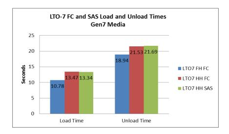
The IBM LTO-7 tape drive has good load performance for all form factors, generation media and interface types. The time to unload a cartridge is faster for the full height form factor drives for both gen 7 and gen 6 media.
